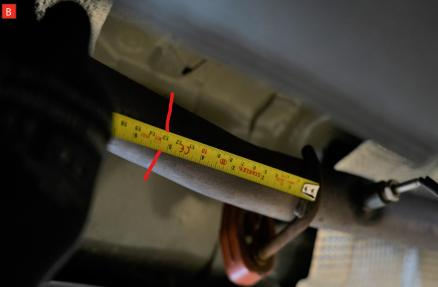
To remove the original exhaust the system requires cutting in two places.
